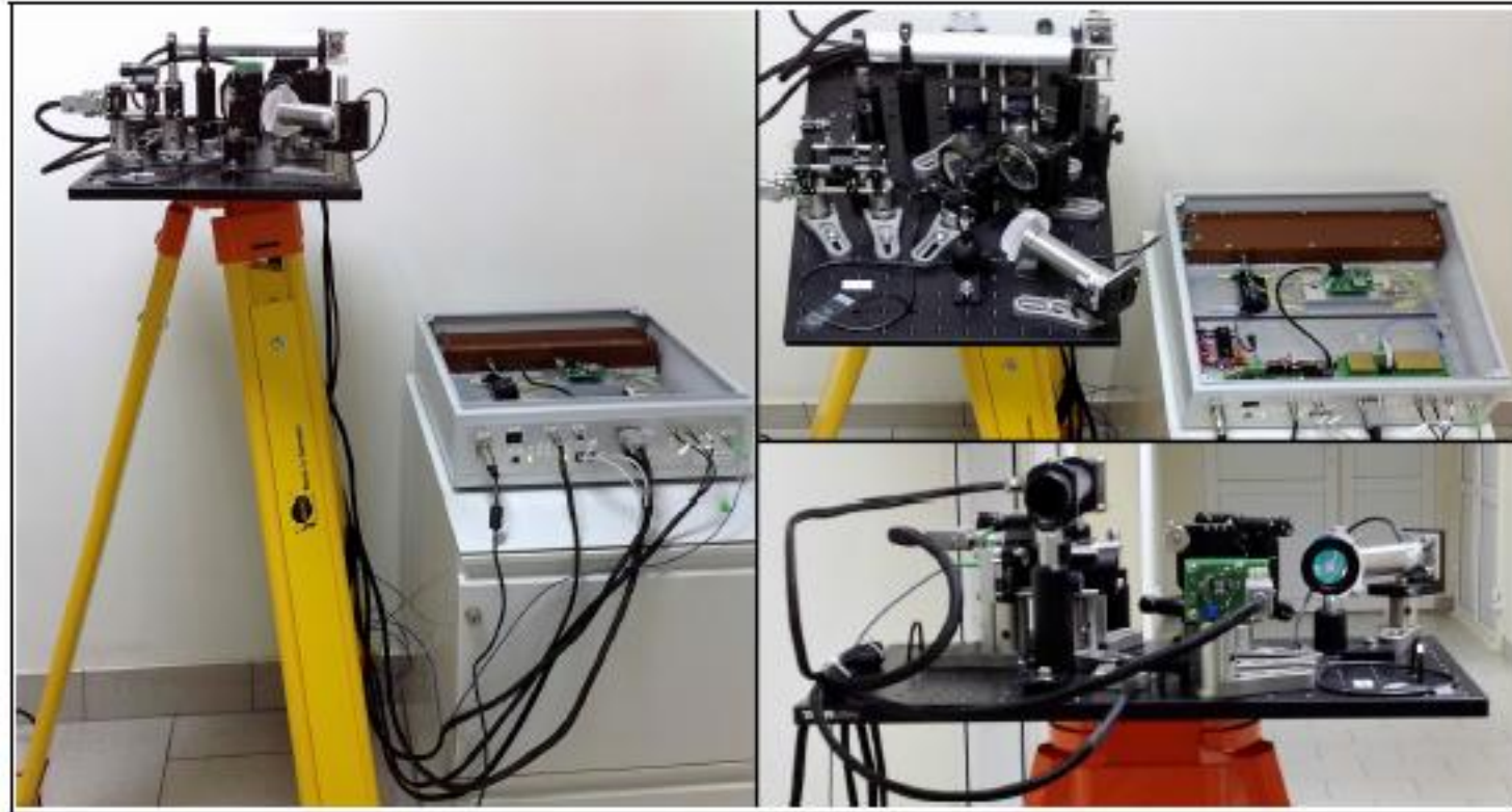
FIG. 3: Station Alice: a tripod tracking platform and a box with all electronics.
